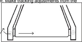
depending on use and walking/running characteristics. Some users will effect tracking differently. Expect to make adjustments as required to center the tread-belt. Adjustments will become less of a maintenance concern as the belt breaks in over time. Proper belt tracking is an owner responsibility common with all treadmills.
